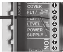
Chlorine probe detector FL2 (rotameter) ③ black ⑤ brown ⑥ blue
