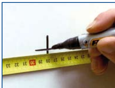
Mark the dimensions of the motor flange.
