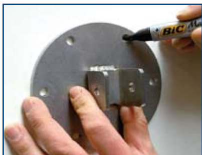
Mark the drill holes for the bearing flange.
