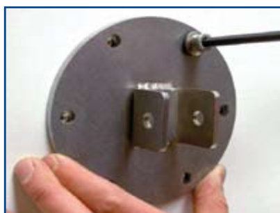
Secure the flange on the bearing side using the short M8 bolts with neoprene washers.
