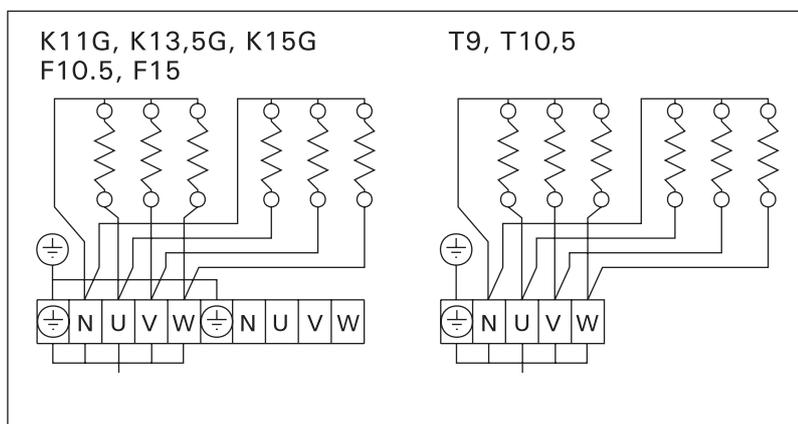
Figure 4. The heater's electrical connections
