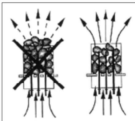
Figure 1. Piling of the sauna stones
