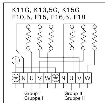
Figure 5. The heater's electrical connections in two groups
