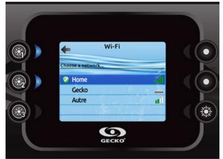
For the Wi-Fi menu to appear in the Settings menu your in.touch module must be equipped with software version 11.00 or higher. This menu allows you to connect your in.touch module to a Wi-Fi network or to change its network.
