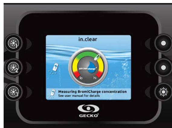
When BromiCharge is added the indicator will move slowly to the right. When water is added to the spa the indicator will move to the left. To obtain a good level of BromiCharge, start the pumps and add the specified amount of BromiCharge\*\* and allow 5 minutes for the indicator to adjust before adding more.
