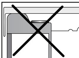
in.k800 must be installed on the outside edge of the hot tub, so that it is not subject to moisture trapped by the cover.
