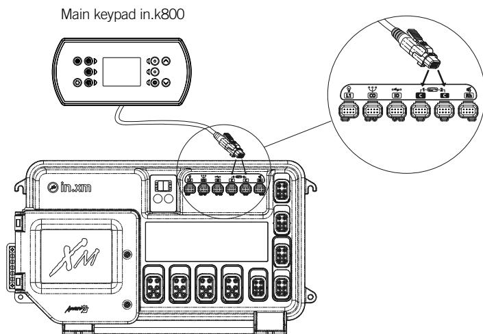
To connect the in.k800 keypad, simply insert its in.link connector into the appropriate keypad connector of the pack enclosure (as illustrated).
