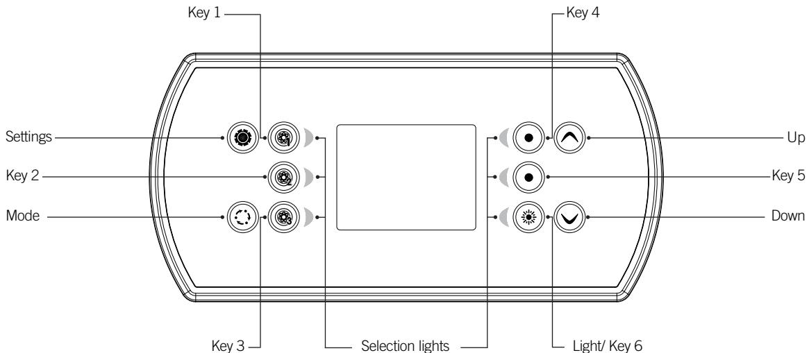
\* Functions for keys 1 to 5 will depend on your system's low level configuration.
