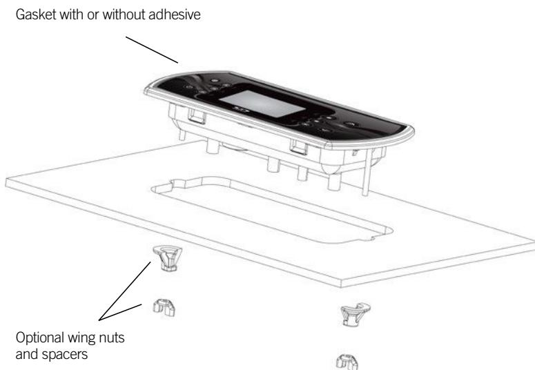
To install the in.k800, use the drilling template provided in this section.
