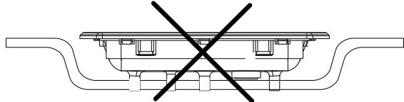
The back of the in.k800 should not be enclosed where water can gather, but instead cut out.
