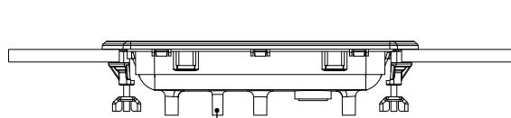
Vent hole on back of keypad should not be blocked.
