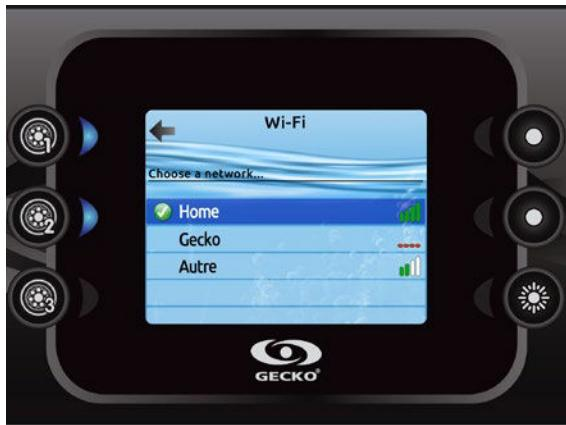
Once the in.touch module is connected to a Wi-Fi network a green check mark will appear in the Wi-Fi menu, and the network name will appear in the *Settings* menu.
