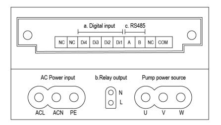
a. **Digital Input:** To enable external speed control, connect one of the digits from Di1/2/3/4 to COM. See schematic as below:
