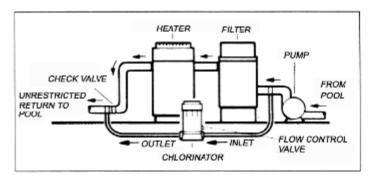
**NOTE**: Never install chlorine feeder directly into copper plumbing as pipe damage may occur. If you have brass or bronze backwash valves, or other sensitive metallic components, consult your dealer for precautions or recommendations for your particular system.
