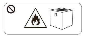
b. The installation can't be in a closed environment or indoors, and must be kept well ventilated.
