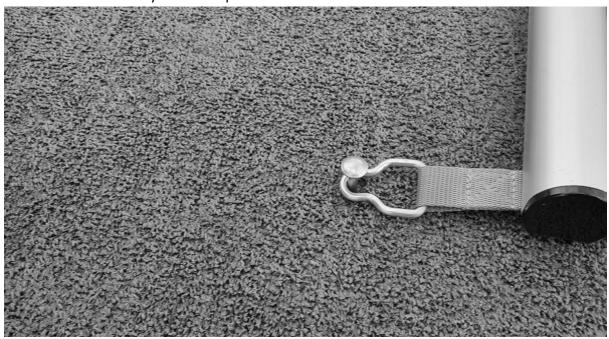
7. Set the pull-out belt attachment in the middle position (fastening with slot), tighten the locking screw with a 2 mm Allen key and then attach the pull-out belt to it.
