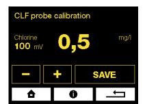
**Do not calibrate the probe** until the water in the pool is perfectly mixed and the value on the ASIN AQUA display is stable.
