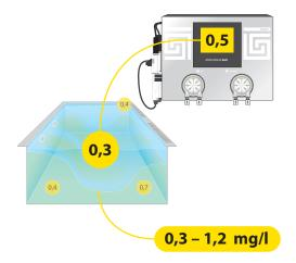
Perform the calibration with a chlorine concentration in the range of  $\bf 0.3$  -  $\bf 1.2$  mg /  $\bf I$ , and with a measured value equal to or greater than the required value.
