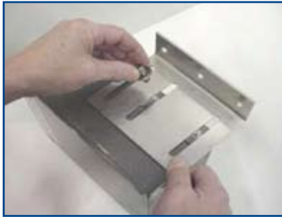
Fit motor bracket on motor.
