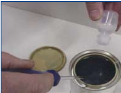
Add hardener to resin and mix well.
