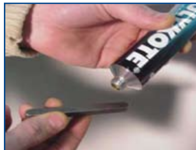
Grease key and fit in the drive motor.
