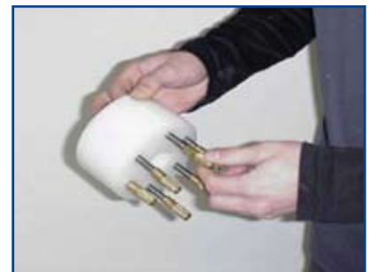
Place plugs on tap bolts and tighten to expansion slug.
