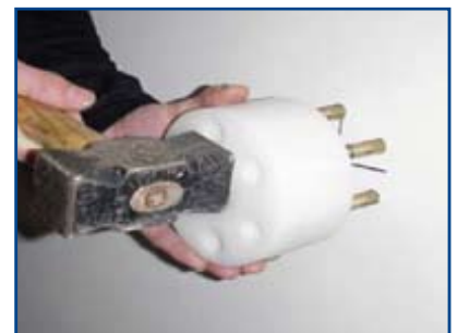
Fit bearing block.
