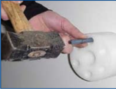
Use a punch to drive tap bolts completely into the hole.
