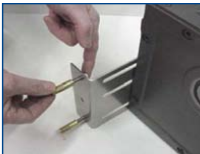
Screw tap bolt + plug together on motor bracket and apply grease in the motor bush.
