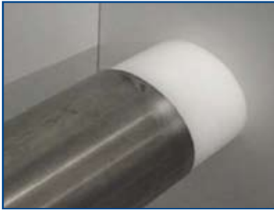
Slide tube into bearing block.
