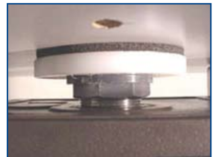
Place motor flush against threaded end to prevent movement of seal and then secure motor bracket on wall side and motor side.
