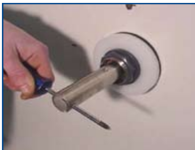
TIP! Use drilled hole at keyway to move shaft.
