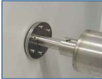
Slide drive shaft into coupling bush of tube.
