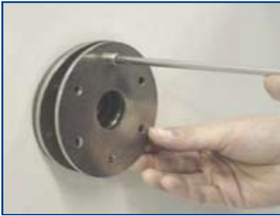
Remove liner flange.
