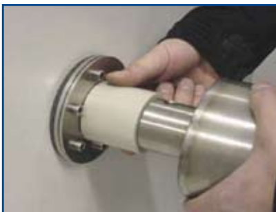
Slide out drive shaft, fit spacer bush in between and secure with M10 bolt.
