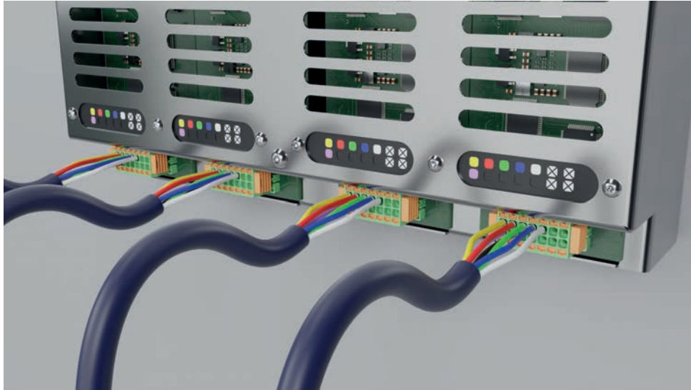
3. Connect the 7-core cables from the underwater lights to the PSU Ensure they are inserted into the correct ports.
